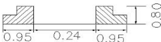
Recommended soldering pad design
